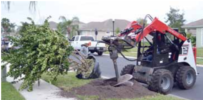
Pictured above, an Arbor-Tech employee drills a hole using a Bobcat digger. Below, workers loosen dirt and enlarge the hole to correct size.
