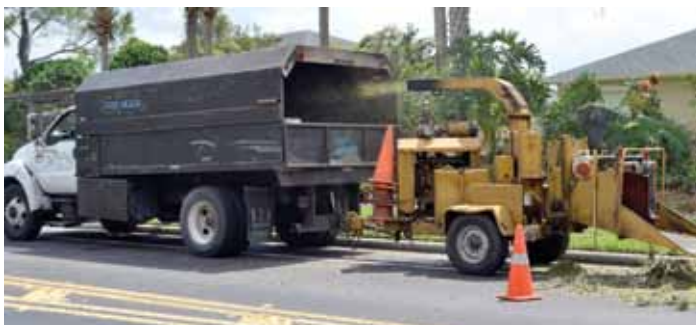
The truck and grinder that Mid-Florida used to ground up the tree limbs as soon as they were removed from the trees on Summergate Blvd.
