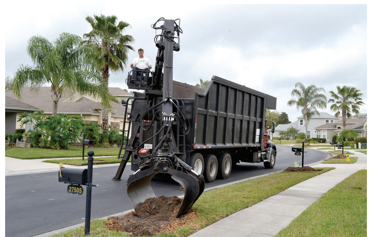
Arbor-Tech employee uses the bucket on the grapple truck to remove debris from the oak tree cut down and dig deep enough to plant sod.
