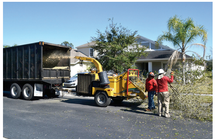
Arbor-Tech employees put the limbs of oak trees in a grinder which changes them to mulch and blows it into a truck.
